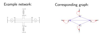
The incidence matrix and the Kirchhof laws, together with the 8th order models of the synchronous generators provide a port-Hamiltonian model of the overall system.
