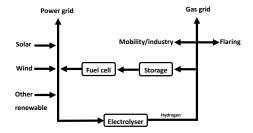
• Presentation tomorrow. Two layer optimization problem: maximize PtG's profit, and DSO's of three grids have to avoid overloading of grids. Builds on Biegel et al. 2012.
