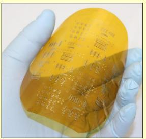
We harness the properties of metal NCs by using nanoimprint lithography to print large-area metamaterials on glass and plastics with widely tailorable optical properties that are used to realize near-infrared optical devices.
