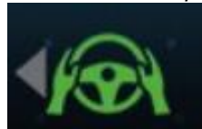
Figure 28 In a Mercedes C-Class, the arrow indicates lane change assistance to the left [ID5289]
