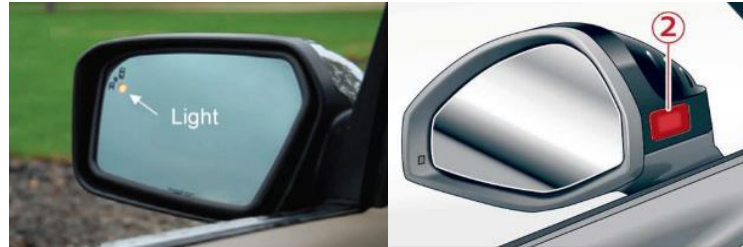
Figure 31 Blind spot information system light in mirror (Ford [ID5270]) and next to the mirror (Audi A5 [ID5290]).
