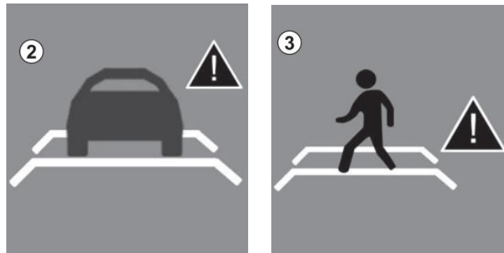
Figure 26 Warning symbol (option 2) for FCW for detected vehicles (left) or detected pedestrians (right) Renault Scenic [ID5363]
