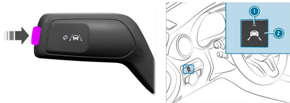
Figure 13 Button to activate Lane keeping System for Ford Focus (left [ID5284]) and Mercedes-Benz S-class (right [ID5289]).
