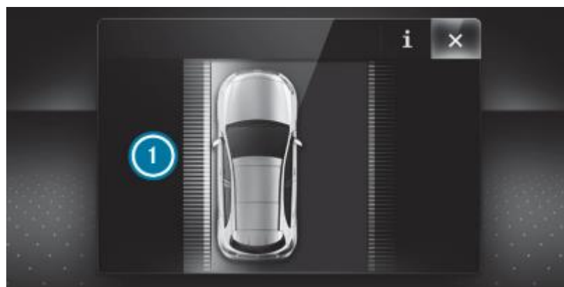
Figure 16 Multifunction display of Mercedes C-Class showing lane-correcting brake application [ID5289].
