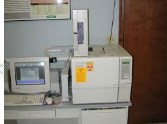
Electron Capture Detector ( ^{63}\text{Ni} )
