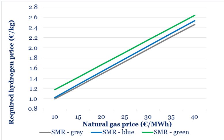
Figure 2.1 Required hydrogen price for SMR in relation to natural gas price, per type
